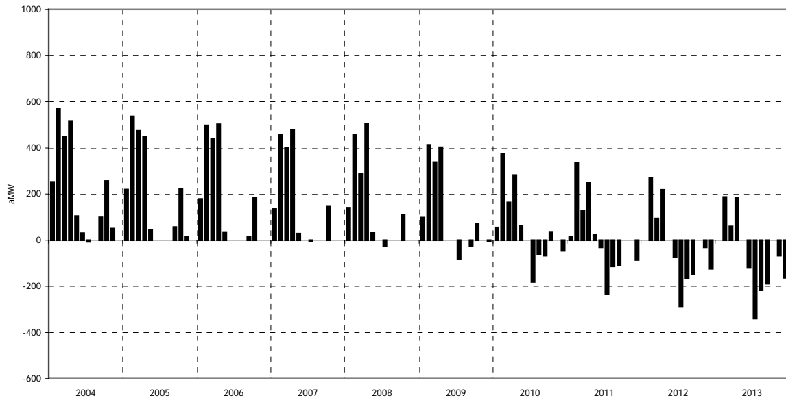
Figure 4 Monthly Energy Surplus / Deficiency 70 th Percentile Water and Load, Existing and Committed Resources
