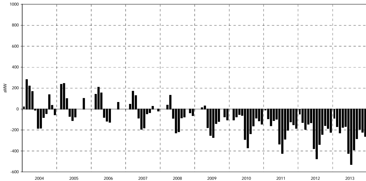
Figure 6 Monthly Energy Surplus / Deficiency 90 th Percentile Water, 70 th Percentile Load, Existing and Committed Resources
