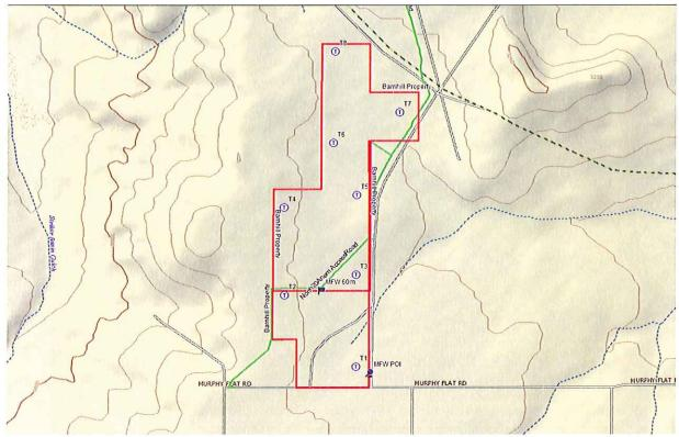
Murphy Flat Wind – Preliminary Turbine Layout 8 Turbines – Clipper Liberty, 2500 kW each, 20MW Total Project Size MFW Point of Interconnection: N 43 deg 11.09277' W 116 deg 28.75851' El 3135 ft WGS84
